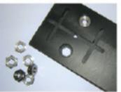
are generally softer than metal, a metal hex insert greatly increases the thread strength and reduces the chances of damage when torque is applied. To insure the hex inserts are installed correctly Technicor machines the hex profile in the plastic part, guaranteeing no misalignment.
