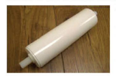
A new product from Technicor can reduce costs and help guarantee food quality. METAL-FREE conveyor rollers are ideal for food-processing areas where metal detectors need to function flawlessly or where wash-down solutions prohibit any metal content. Rollers, bearings, shafts and "hardware" are all plastic. The ball-bearings are fitted with glass balls and nylon or acetal 7/16" hex shafts. Fit them into UHMW slotted side rails and you have a METAL-FREE conveyor!
