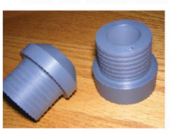
Off-the-shelf fittings are not always suitable. Special features such as threads, collars, flanges, and grooves may be needed to adapt to specific components. Our large CNC lathe can mass-produce such parts up to 4" outside diameter.
